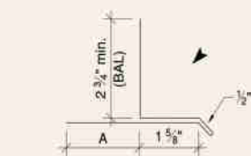
⊛ INDUSTRIAL WINDOW & DOOR FLASHING #106 (A+7"=GIRTH)
